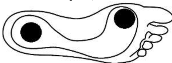
Figure 1. Location of transducers in this development.
